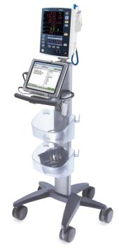
Optional rolling stand features tablet computer mount, bar code scanner cradle and spacious bins.
